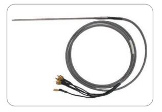
The **Thermometrics Type S/AS/ES** temperature standards consist of ultra-stable thermistor probes assembled into thin wall stainless steel housings with shielded extension leads. The thermistors used receive special processing to ensure long term stability. All thermistor temperature standards are ruggedly constructed and are suitable for liquid immersion.
