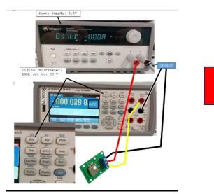
This sensor is not revers or over voltage protected. Be sure of setup before applying
